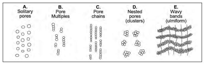
Figure 6. Vessel (pore) arrangement
