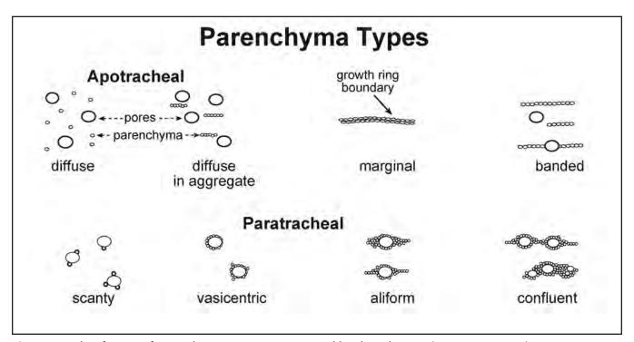
Figure 7. Classification of parenchyma arrangements around hardwood pores. (cross-section view)
