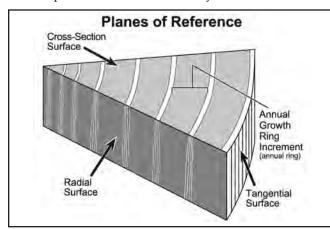
Figure 1. Three-dimensional orientation of wood material.
