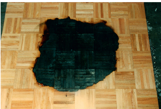
Figure 19 A 'puddle-shaped' pattern, similar to one that was attributed to the burning of a puddle of ignitable liquid. Actually, this pattern was caused by the burning of a cardboard box. Copyright 2012 from Scientific Protocols for Fire Investigation, 2nd Edition by John J. Lentini. Reproduced by permission of Taylor and Francis Group, LLC, a division of Informa plc.
