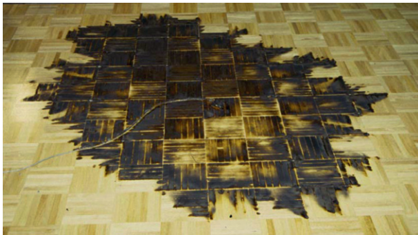
Figure 20 A fire pattern on a parquet floor that was caused by the burning of 1 l of gasoline.
