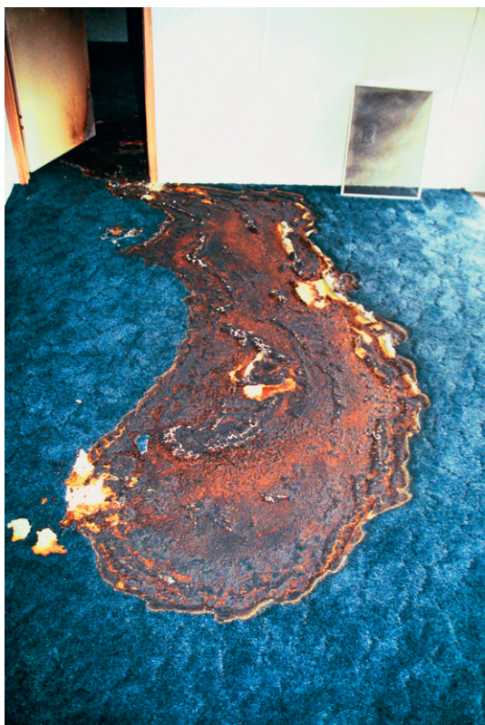
Figure 15 Irregular pattern caused by the burning of a medium petroleum distillate on a carpet. This is a rare instance where the cause of the pattern can be interpreted as having been caused by ignitable liquids on the basis of appearance alone. Copyright 2012 from Scientific Protocols for Fire Investigation, 2nd Edition by John J. Lentini. Reproduced by permission of Taylor and Francis Group, LLC, a division of Informa plc.
