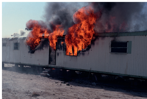
Figure 23 Although this fire started in the kitchen at the left, the living room at the right exhibited far more damage. Copyright 2012 from Scientific Protocols for Fire Investigation , 2nd Edition by John J. Lentini. Reproduced by permission of Taylor and Francis Group, LLC, a division of Informa plc.
