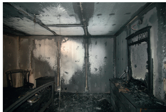
Figure 22 Clean burn resulting from a fire that burned for approximately 2 min beyond flashover. The V-shape developed from the top downward. The fire originated between the bed in the chair. Photo courtesy of ATF Fire Research Laboratory and Steven W. Carman, Carman Fire Investigations, with permission.
